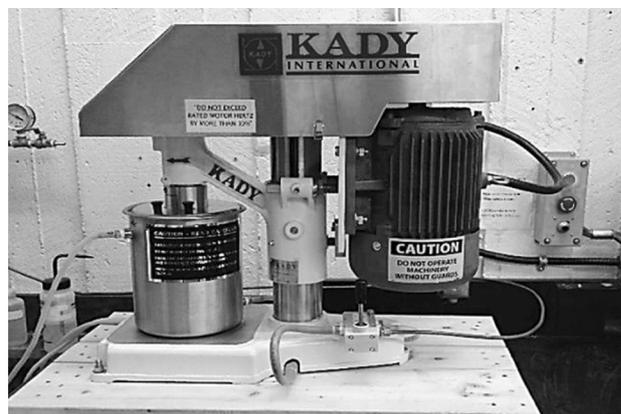
**Fig. 1** Kady<sup>®</sup> International rotor–stator dispersion mill used for preparing AgNP suspensions
